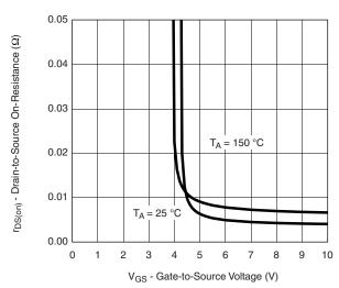
On-Resistance vs. Gate-to-Source Voltage
