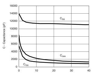
V<sub>DS</sub> - Drain-to-Source Voltage (V) **Capacitance**
