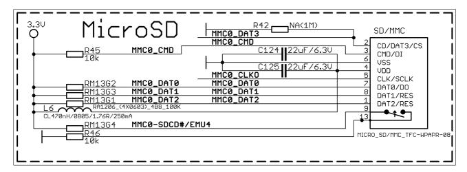
This slot is typically used for booting the OS, due to the larger capacities of the microSD cards (compared to SD or MMC cards). It is suggested to have an SD card with a proper Linux. It is recommended to use class 10 (10MByte/sec) card for faster read/write operations, since lower class cards (especially higher capacity ones) might slow down the whole system.
