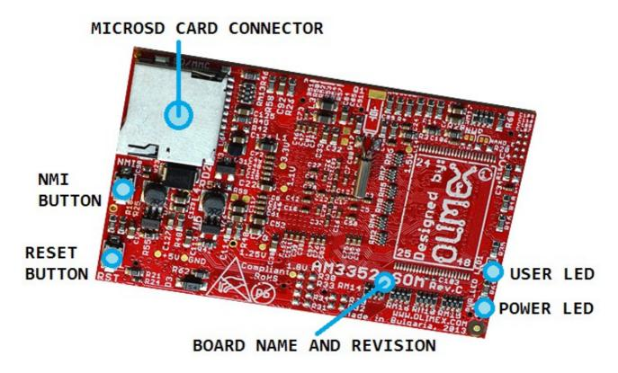
The power LED indicates whether the board is powered properly. It is not connected to a processor pin.
