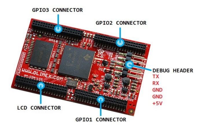
The four plastic connectors (AM\_CON-LCD; AM\_CON-GPIO1; AM\_CON-GPIO2; AM\_CON-GPIO3) have 0.05" step between the pinholes. These connectors are typically used to connect to AM3352-SOM-EVB.
