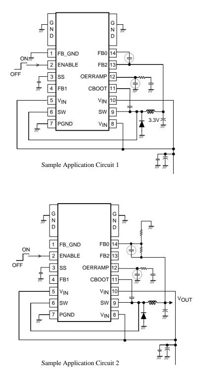
\*The capacitor between the FB0 and V<sub>OUT</sub> pins and capacitor between the OERRAMP pin and GND (the capacitors shown inside the broken lines in the diagram) are used for phase compensation. Their capacitance is intended to stop oscillation when oscillation is caused by the status of the output capacitor. As such, they can be left open under normal circumstances.
