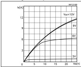
Figure 5. Transfer characteristics
