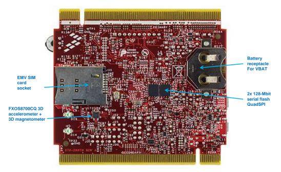
Figure 2. Back side of TWR-KL82Z72M module
