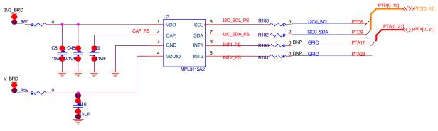
Figure 8. Pressure sensor connection
