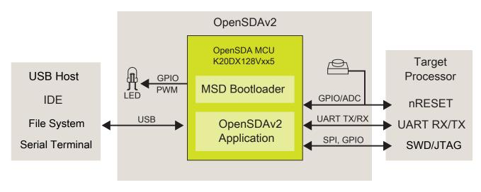
Figure 5. OpenSDAv2 high-level block diagram
