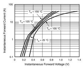
Fig. 3 - Typical Instantaneous Forward Characteristics
