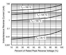
Fig. 4 - Typical Reverse Characteristics
