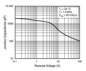
Fig. 6 - Typical Junction Capacitance
