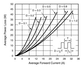
Fig. 2 - Forward Power Dissipation Characteristics
