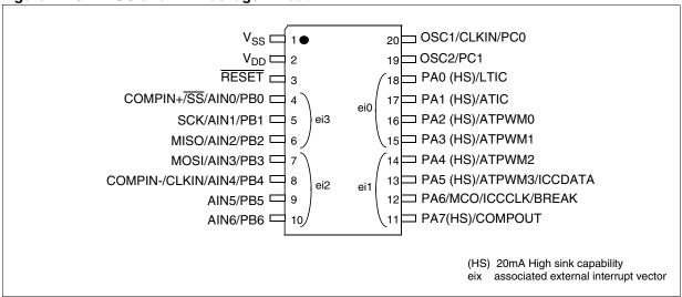
Figure 3. 20-Pin QFN Package Pinout
