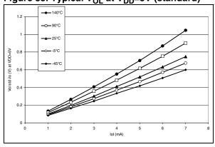
Figure 84. Typical V<sub>OL</sub> at V<sub>DD</sub>=2.7V (Port C)
