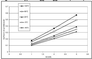
Figure 86. Typical V<sub>OL</sub> at V<sub>DD</sub>=5V (Port C)
