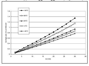
Figure 90. Typical V<sub>OL</sub> vs. V<sub>DD</sub> (standard I/Os)
