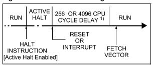
Figure 28. ACTIVE-HALT Mode Flow-chart
