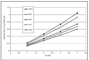
Figure 101. Typical V<sub>DD</sub>-V<sub>OH</sub> at V<sub>DD</sub>=5V (Port C)
