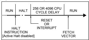
Figure 26. HALT Mode Flow-chart
