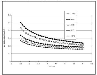
Figure 91. Typical  $V_{OL}$  vs  $V_{DD}$  (High-sink)
