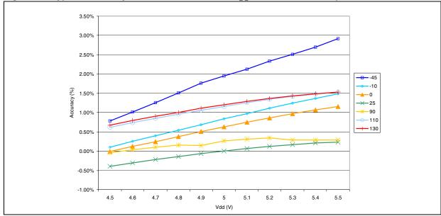
Figure 67. Typical RCCR0 vs  $V_{DD}$  and Temperature
