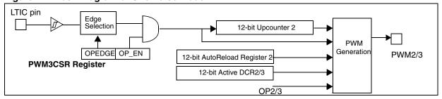
Figure 48. One Pulse Mode and PWM Timing Diagram
