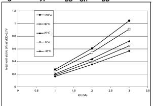
Figure 94. Typical  $V_{DD}$ - $V_{OH}$  at  $V_{DD}$ =3.3V
