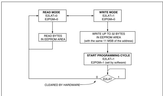
Figure 9. Data E<sup>2</sup>PROM Write Operation
