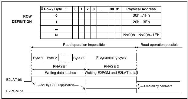
**Note:** If a programming cycle is interrupted (by a reset action), the integrity of the data in memory is not guaranteed.
