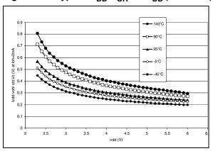
Figure 103. Typical  $V_{DD}$ - $V_{OH}$  vs.  $V_{DD}$  (High Sink)
