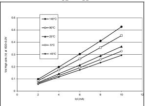
Figure 89. Typical  $V_{OL}$  at  $V_{DD}$ =5V (High-sink)
