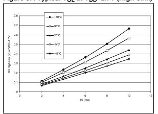
Figure 88. Typical V<sub>OL</sub> at V<sub>DD</sub>=3.3V (High-sink)
