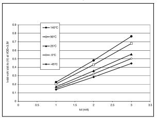
Figure 95. Typical V<sub>DD</sub>-V<sub>OH</sub> at V<sub>DD</sub>=5V
