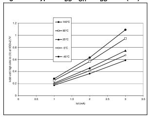
Figure 97. Typical  $V_{DD}$ - $V_{OH}$  at  $V_{DD}$ =3.3V (HS)
