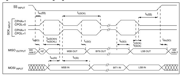
Figure 109. SPI Master Timing Diagram 1)
