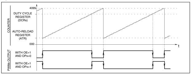
Figure 39. PWM Signal from 0% to 100% Duty Cycle
