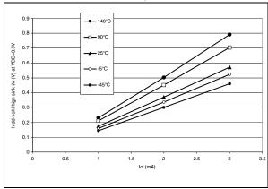
Figure 98. Typical  $V_{DD}$ - $V_{OH}$  at  $V_{DD}$ =5V (HS)
