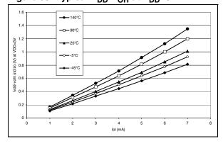
Figure 96. Typical V<sub>DD</sub>-V<sub>OH</sub> at V<sub>DD</sub>=2.7V (HS)
