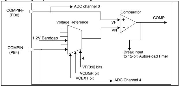
Figure 62. Analog Comparator
