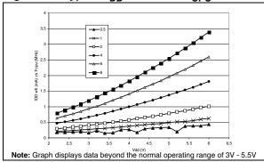
Figure 76. Typical  $I_{DD}$  in SLOW-WAIT vs.  $f_{CPU}$
