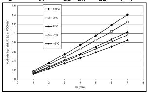
Figure 99. Typical V<sub>DD</sub>-V<sub>OH</sub> at V<sub>DD</sub>=2.7V (Port C)
