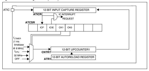
Figure 44. Input Capture timing diagram
