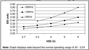
Figure 74. Typical I<sub>DD</sub> in WAIT vs. f<sub>CPU</sub>
