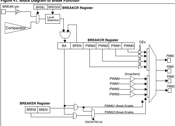
Figure 41. Block Diagram of Break Function
