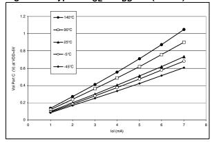
Figure 87. Typical  $V_{OL}$  at  $V_{DD}$ =2.7V (High-sink)
