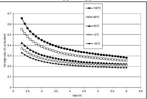
Figure 92. Typical V<sub>OL</sub> vs V<sub>DD</sub> (Port C)
