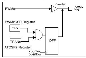
The Data Flip Flop (DFF) applies the polarity inversion when triggered by the counter overflow input.
