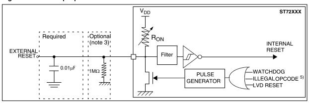
Figure 106. RESET pin protection when LVD is disabled.<sup>1)</sup>
