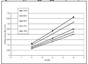
Figure 85. Typical V<sub>OL</sub> at V<sub>DD</sub>=3.3V (Port C)
