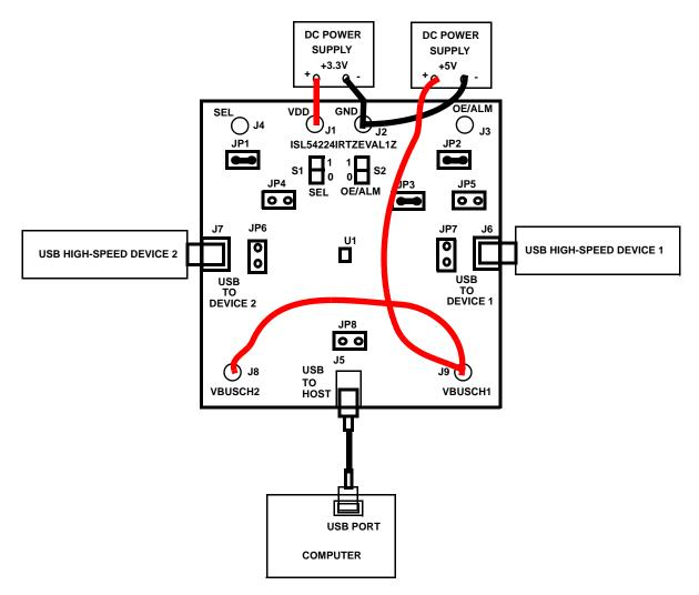
Note: For Device 1 to get VBUS from the computer through the J5 connector, disconnect the 5V supply from J9 and populate jumper JP5. For Device 2 to get VBUS from the computer through the J5 connector, disconnect the 5V supply from J8 and populate jumper JP4.
