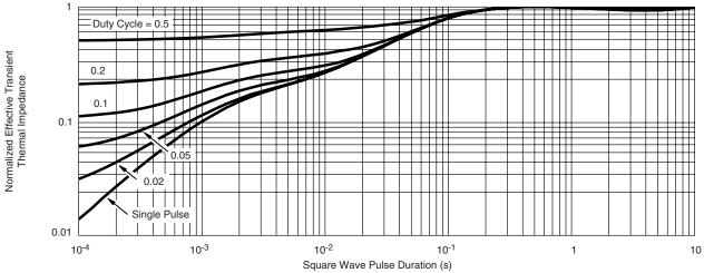
Normalized Thermal Transient Impedance, Junction-to-Case
