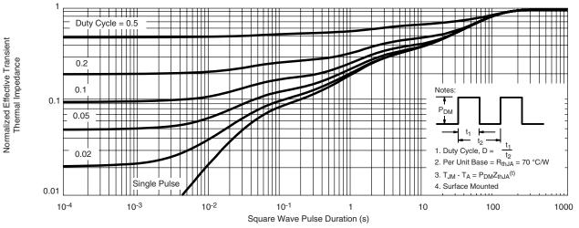
Normalized Thermal Transient Impedance, Junction-to-Ambient
