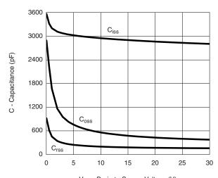
V<sub>DS</sub> - Drain-to-Source Voltage (V) Capacitance
