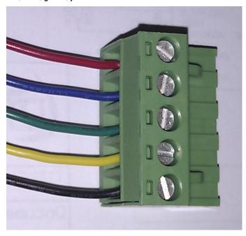
Figure 8 – BLDC motor hall sensor cables
