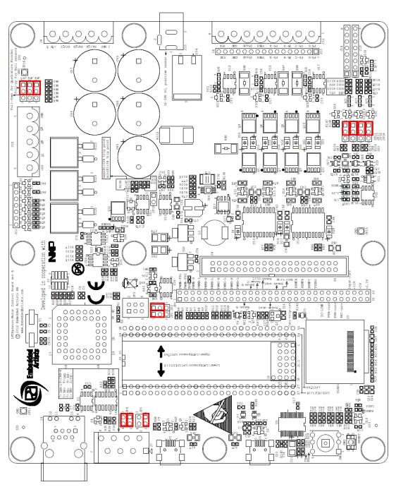
Figure 5 - Default jumper positions, rev B hardware
