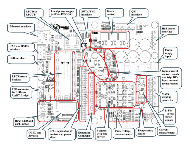
Figure 2 – LPCXpresso Motor Control Board Detailed Overview, rev B
