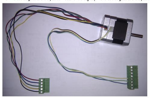
Figure 7 – BLDC motor with screw connectors
