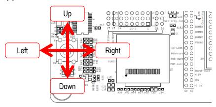
Figure 4 - LPCXpresso Motor Control Board Joystick Directions, rev B
