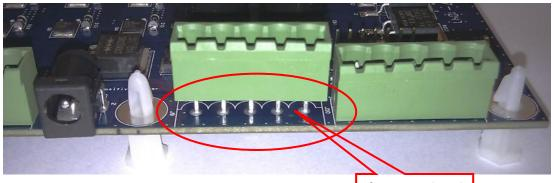
Figure 19 – Screw Connector Housing
