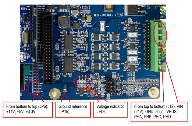
Figure 20 - Measurement Pad Locations, rev A board
